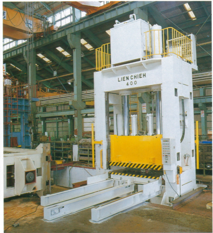
400 TON TRYOUT-DIE SPOTTING PRESS EQUIPPED WITH 180 DEGREE SLIDE TILT SYSTEM FOR IN PRESS DIE WORK.
