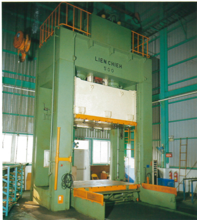
500 TON TRYOUT-DIE SPOTTING PRESS EQUIPPED WITH 180 DEGREE SLIDE TILT SYSTEM FOR IN PRESS DIE WORK.
